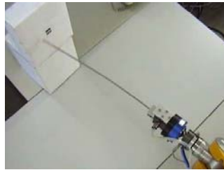
Figure 8. Experimental set-up. The DLO is grasped by pneumatic jaws and the robot conducts an adjustment motion to reduce vibration before inserting into a hole.
