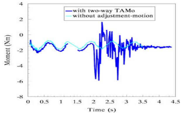
Figure 9. Measured moment  $M_y$  during the force/torque sensor-based adjustment-motion process
