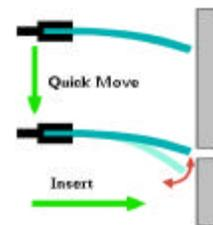
Figure 1. The vibration caused by a quick operation results in uncertainty and failure, e.g. when inserting a DLO into a hole.
