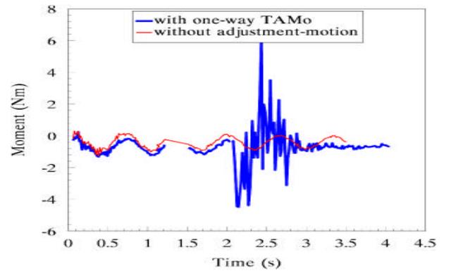
Figure 8. Measured moment  $M_y$  during the force/torque sensor-based adjustment-motion process
