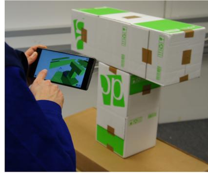
**Figure 3** Acquisition of static obstacles through a smartphone.
