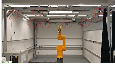
**Fig. 3.** Multi-camera system with eight consumer-grade Logitech C930e cameras (red circles) monitoring the workspace.
