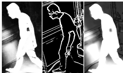
Fig. 3. Left to right: per-pixel probabilistic segmentation after first stage, edge image, spatially optimized segmentation with reduced artifacts.
