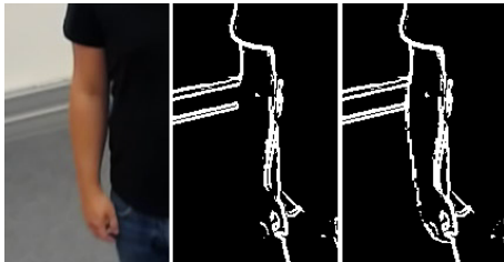
Fig. 2. Left to right: Input color image, output of a basic Sobel Filter, output of our modified Sobel Filter with improved edge detection.
