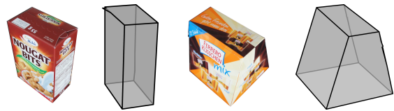
Figure 5: Boundary representation models of two example objects as reconstructed in the offline step of error handling.
