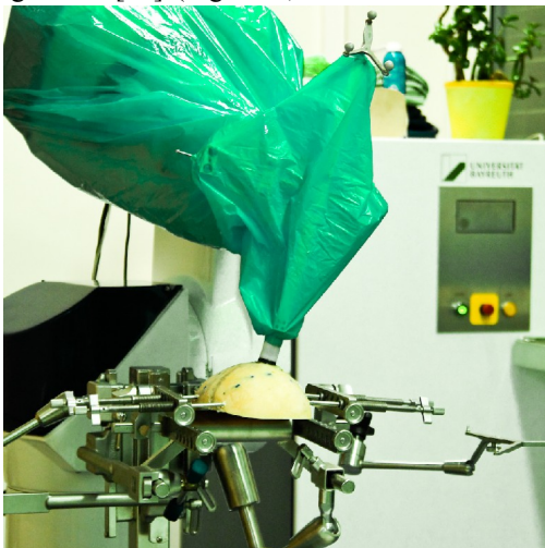
Figure 6: The robot executing the previously demonstrated, post-processed ultrasound scan path on a human specimen.
