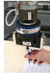
Fig. 7: The user grabs the pen and moves the robot.
