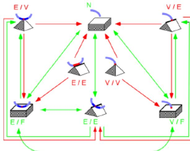
Figure 1: All single contact state transitions between a DLO and its convex polyhedral environment. Initiated transitions (grey); spontaneous transitions (black)<sup>1</sup>
