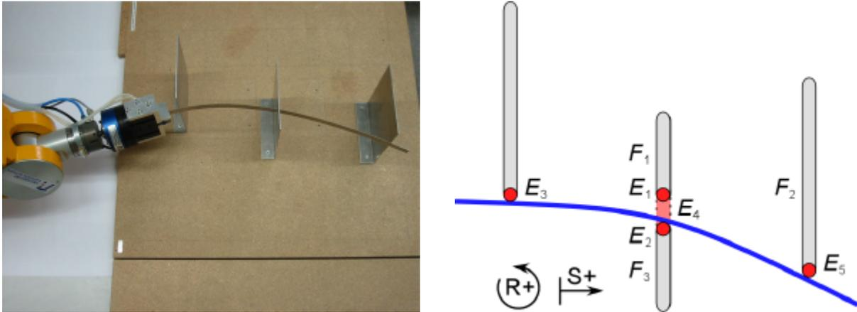
Figure 2: Target situation of leaf spring assembly: Overview (left); Horizontal section with designation of the involved faces and edges. (right)
