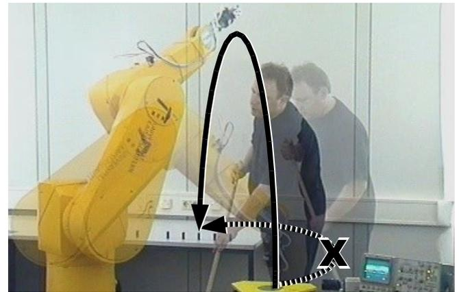
Fig. 6: Illustration of the already implemented free gross motion: Whole arm collision detection in conjunction with evasive movement based on the difference image method implemented by [4] (but without distance-controlled velocity).
