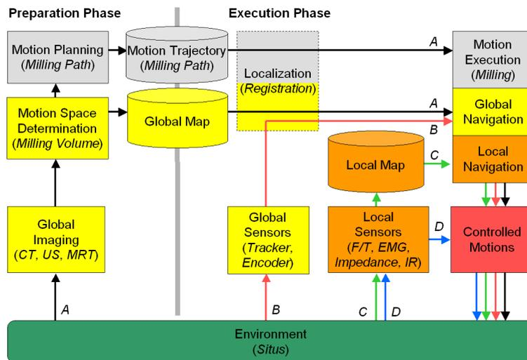
Figure 2: General navigation system architecture including the four navigation principles (A through D)
