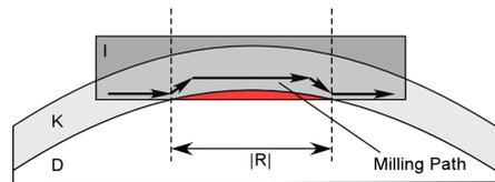
Figure 1: Conservative path modification, lifting miller over critical regions (*I* implant, *K* bone, *D* dura/brain,  $|R|$  extent of critical region)
