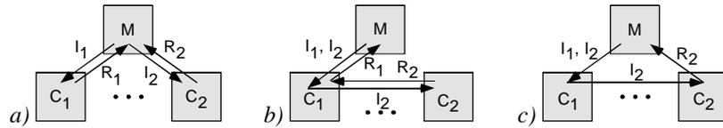
Figure 3: Three types of communication methods between single components: a) standard client/server calls, b) cascade client/server calls, c) instruction chains
