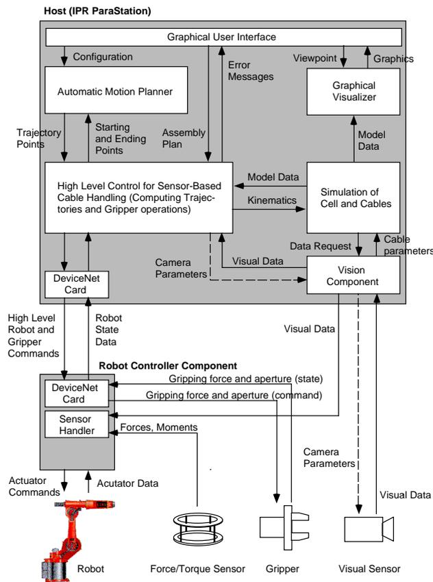
Figure 4: Location and interaction of the components of the example robot system
