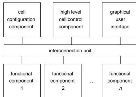
**Figure 1: Concept for the parallel robot control architecture consisting of multiple components and an interconnection unit**
