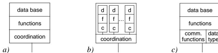
**Figure 2: Different views of the component structure: a) basic parts of a component, b) component with subcomponents for parallel processing, c) component with coordination part split up in communication functions and data types.**
