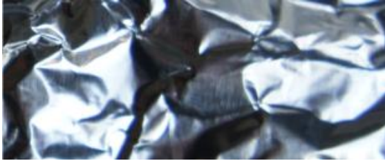
Figure 5 Example of a crinkled aluminum foil (ca. 15 x 20 mm) leading to sensor misdetections in a distance of ca. 1700 mm.
