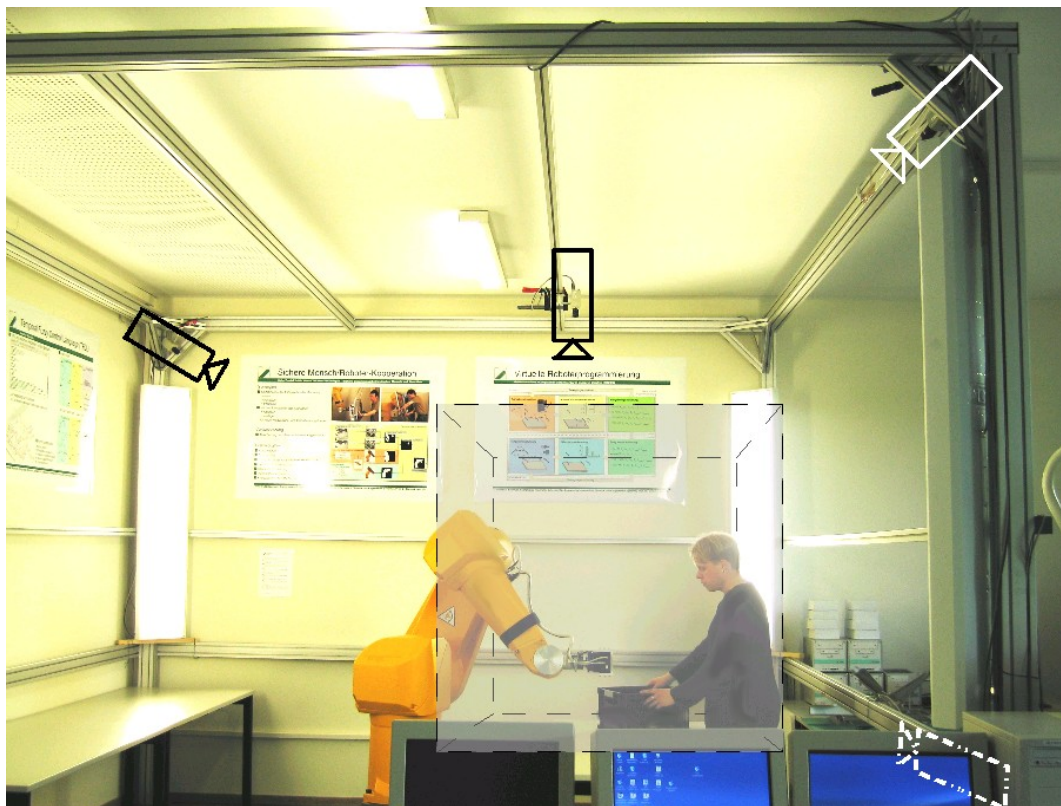
Figure 1: Work cell surveilled by four cameras (indicated by icons). The transparent cube indicates the surveilled space.
