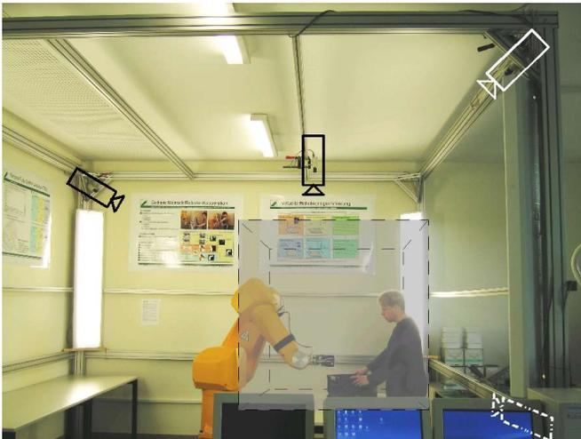
Fig. 5: Prototype system. Work cell with robot and human worker carrying a box. The cameras are indicated by icons (the bottom right one is hidden). The supervised workspace is indicated with a dashed transparent cube.
