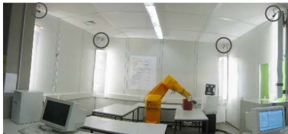
Figure 1: View of the realized prototype system comprising four cameras (black circles)
