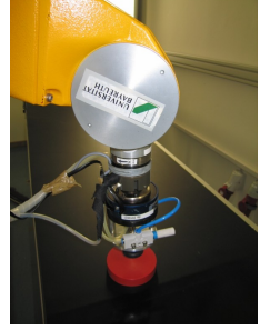
Figure 3: Setup of the second experiment. The vacuum gripper grasps the disk at specified offsets from the center and measures the forces and torques for each position. Based on this information the drift compensation function is approximated using a Householder approximation and a MLP neural network.
