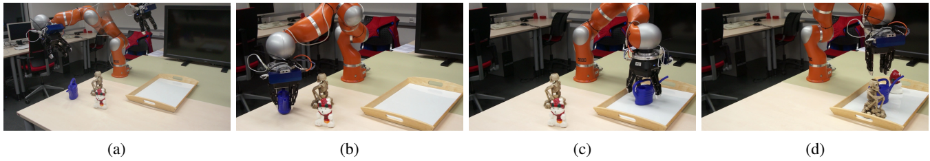
Fig. 4: Snapshots of the example program: (a) sensor based reconstruction, (b),(c) automatic order of execution, evaluation of the object, picking and placing, and (d) the result of the completed program.
